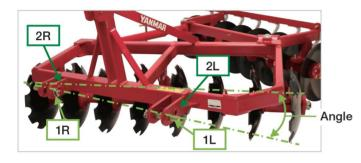
■ Adjustment can be done by changing the pin hole position for the disks in the rear row.
